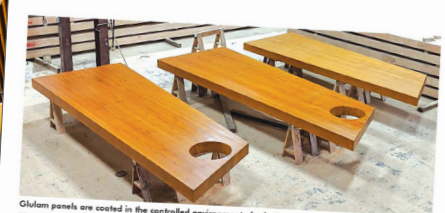
Glulam panels are coated in the controlled environment of a factory setting. Photo courtesy of Samsin Corporation
